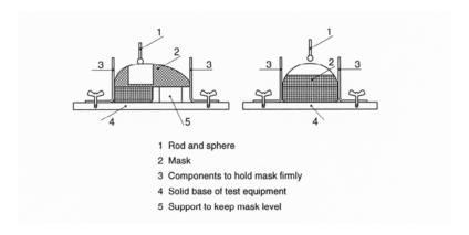
Figure A.2. Method of fixing the mask
