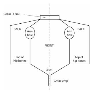
Figure 14. Foil: conductive jacket
