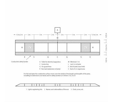
Figure 1. Strip for Semi-Finals and Finals (maximum height 50 cm)
