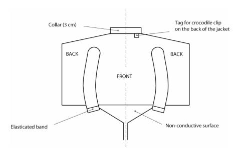
Figure 15. Electric saber conductive jacket
