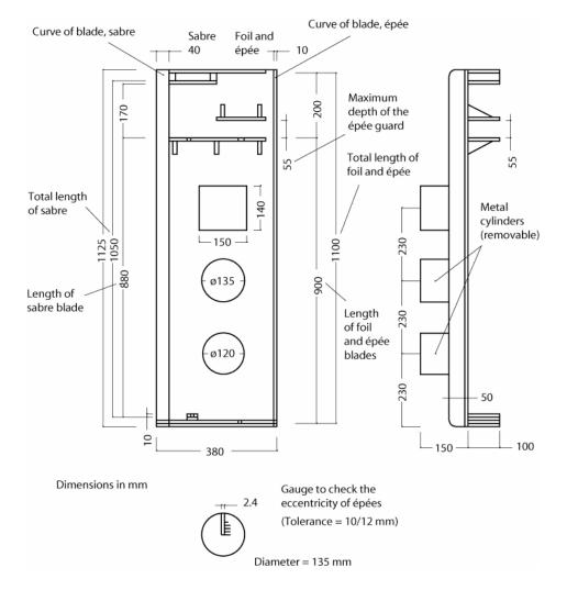
Figure 16. Gauge for checking weapons
