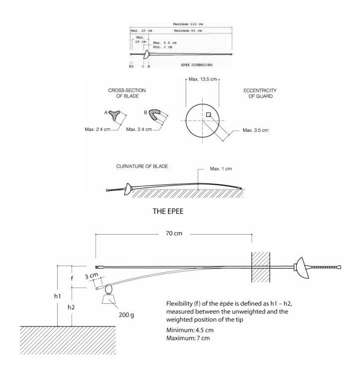
Figure 9. Epee dimensions and flexibility
