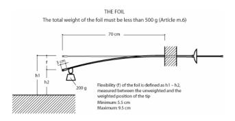
Figure 8. Foil dimensions and flexibility
